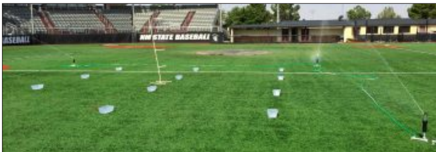
A section of New Mexico State's baseball field, which is artificial turf, was set up with catch cans to make sure the temporarily installed irrigation system reached the whole section equally while measurements were taken twice a day. (Bernd Leinauer photo)
